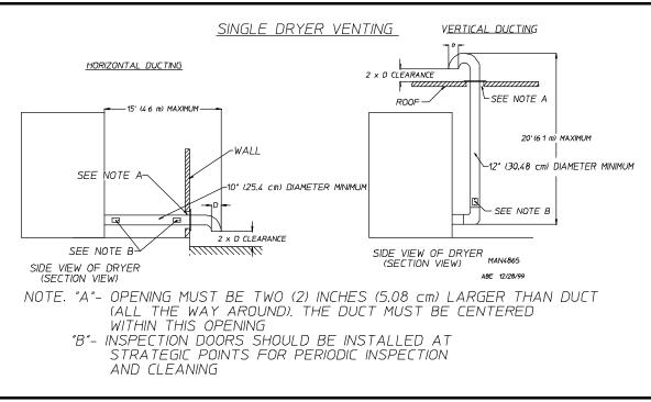
**IMPORTANT:** For extended ductwork runs, the cross section area of the ductwork can only be increased to an extent. When the ductwork approaches the maximum limits noted in this manual, a professional heating, ventilating, and air-conditioning (HVAC) firm *should be* consulted for proper venting information.
